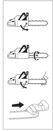
The position of the chain tensioning screw varies from model to model. See the" *What is what*" section to find out where it is on your saw.
